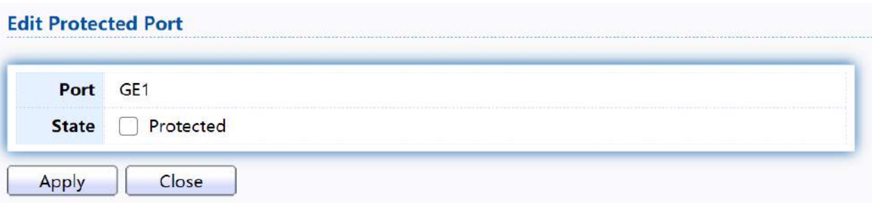
Figure 132 - Security > Protected Port > Edit Protected Port
