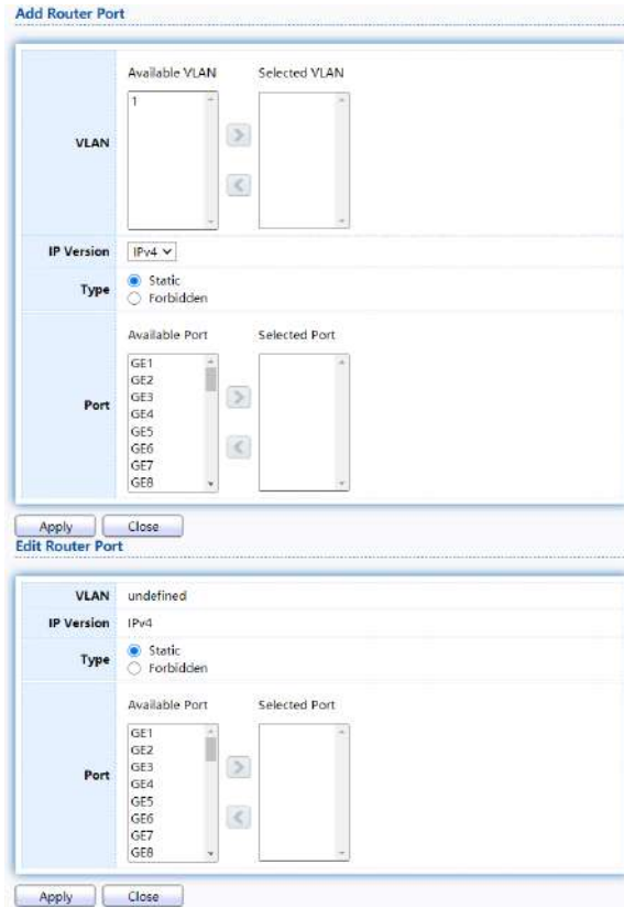
Figure 86 - Multicast > General > Router Port > Add/Edit Router Port
