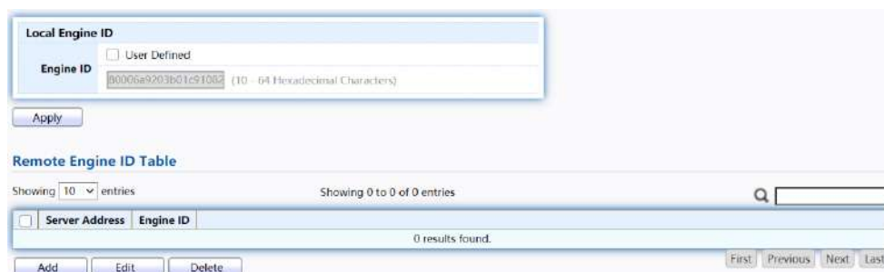
Figure 218 - Management > SNMP > Engine ID
